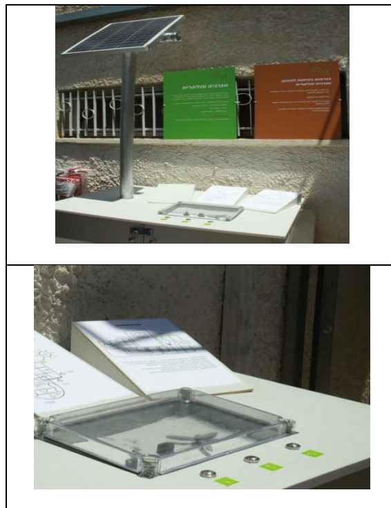
Fig.1. (a) Solar Panel device; (b) Energy Consumers Panel (buzzer, engine and lamp).
